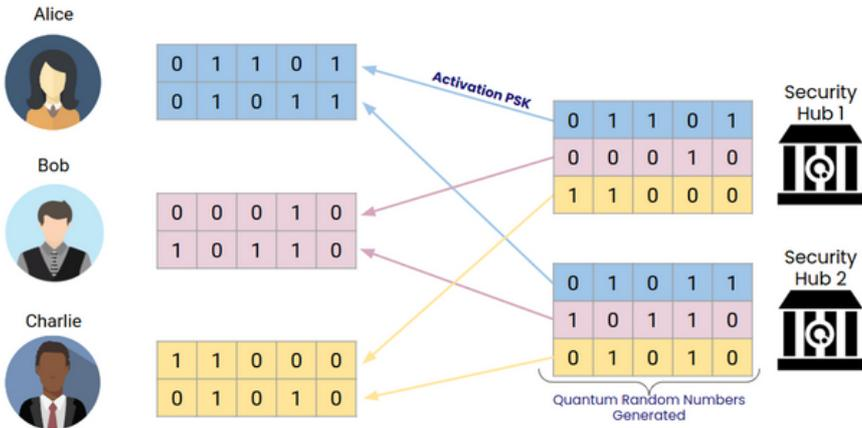
**Set-up.** When a new DSKE client (Alice, Bob or Charlie here) joins the system, each Security Hub generates some new secret random data from a Quantum Random Number Generator. The random data is delivered to the KME using physical tamper-proof devices or other secure channels.
