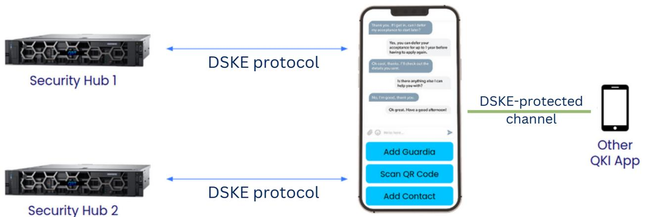
DSKE clients can be easily integrated into endpoint devices such as mobile phones and personal computers. The DSKE clients provide unconditionally secure authentication and encryption, and remove the need to trust any single service provider. DSKE clients can be easily integrated into existing protocols such as TLS/DTLS, WireGuard, IPsec, or any other customized communication protocol with pre-shared key compatibility.
