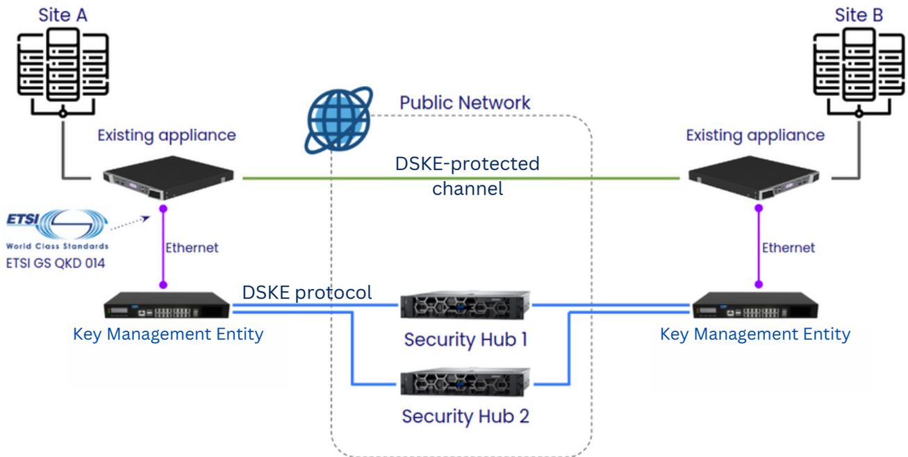
Quantum Bridge's Key Management Entities (KME) connect directly to existing network encryptors and infrastructure. The KMEs key distribution and management is supported by the Security Hubs, which orchestrate and synchronize the generation of secret keys between the KMEs. Once set up, it provides and manages symmetric cryptographic keys on demand, making existing infrastructure quantum-safe and securing it against any weakness or failure in the PKI.
